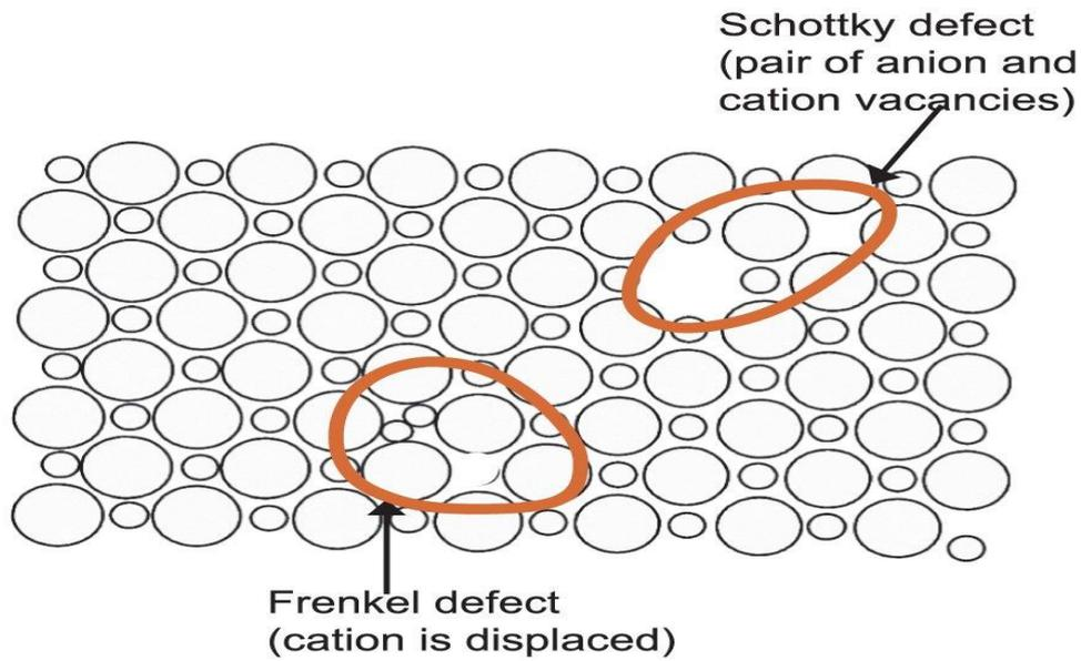
Electrical Balancing Restrictions are also partially responsible for Ceramic Brittleness; Dislocation Movement and Plastic Deformation are minimal.
