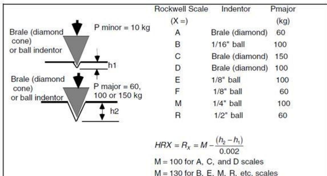
**Figure 1. Rockwell Principle**
